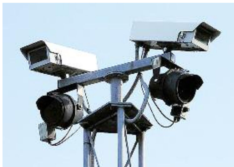
One example of a fixed-mount Automated License Plate Reader (ALPR) system Photo public domain
